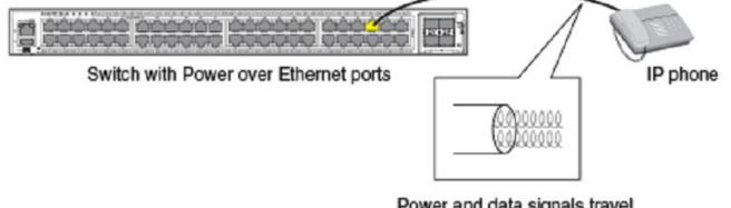
Power and data signals travel along the same pairs of wires at different frequencies.
