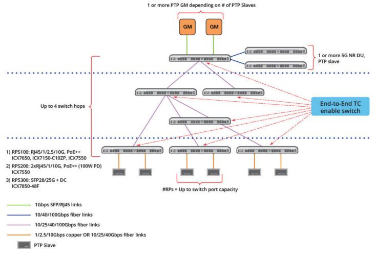
PTP packet prioritization and end-to-end transparent clock is supported by the following RUCKUS devices in both standalone and stacking topology.
