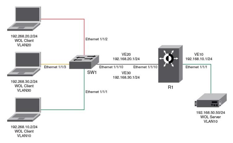
Following is a sample configuration for Wake-On-LAN (WOL) support across different VLANs:
